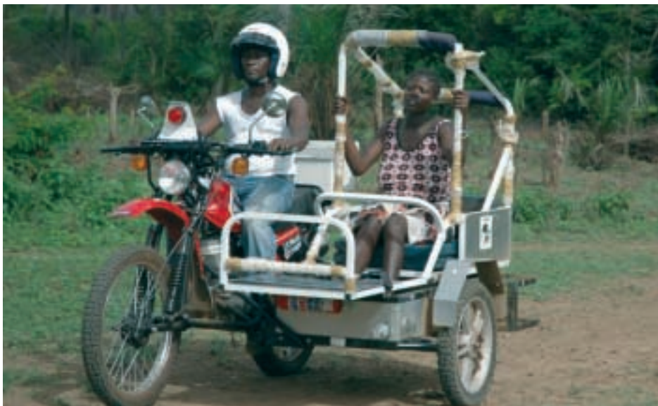
One of our 6 Lifecycles in use – this lady is sitting, but the stretcher can be extended fully if required
